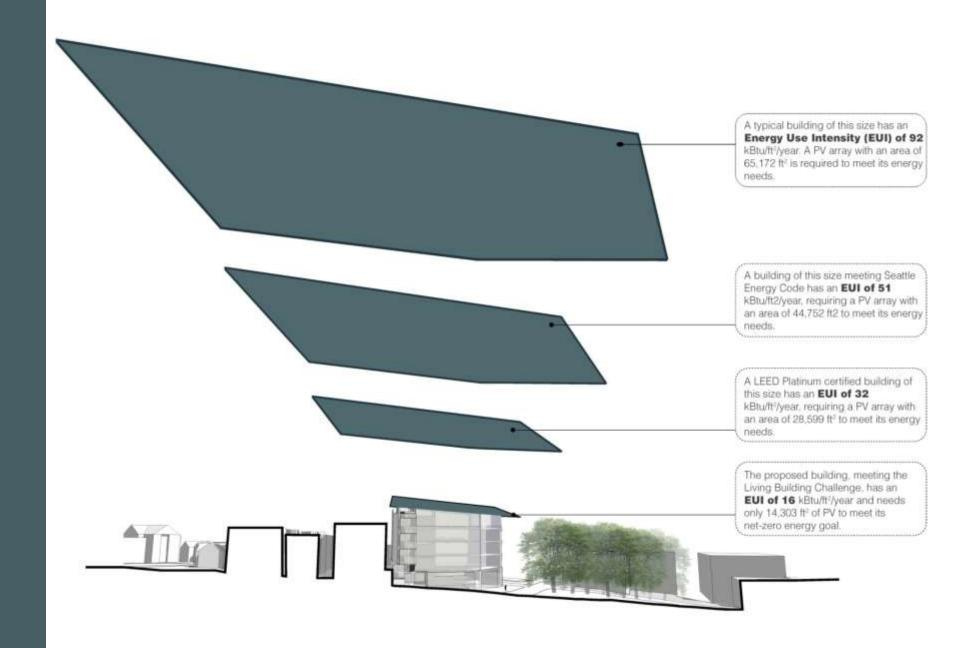
Relative sizes of PV array based on EUI
